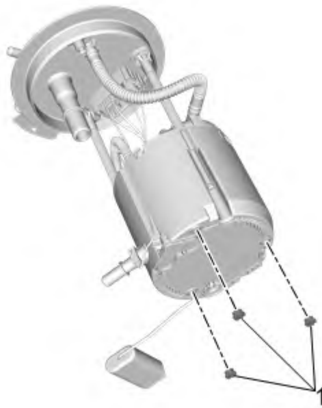
Fig. 83: Inspect Bottom Of Fuel Pump Module For Green Rubber Pads Courtesy of GENERAL MOTORS COMPANY
